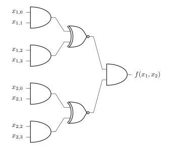
Figure 15: An example of a boolean circuit that could be securely evaluted using Yao's Garbled Circuits.
